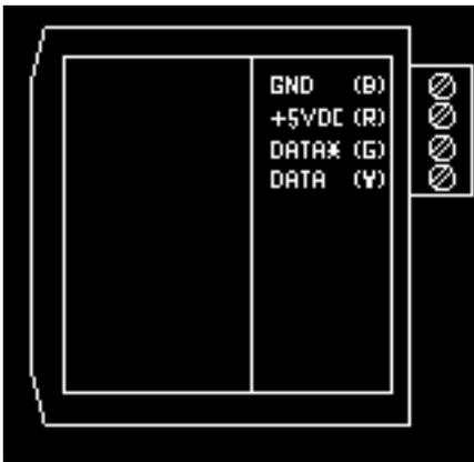
Figure 1A Connections for DIN-191.
