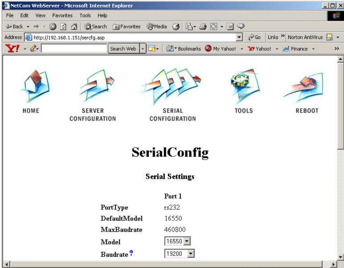
Select the Serial Port Baud Rate, Parity, Data Bits and Stop Bits. The valid data settings for communicating with a DGH module would be: 8-N-1, Odd-7-1, or Even-7-1. For example, if the module is configured for 19.2K Baud and Even Parity then set the Baud Rate to 19.2K, 7 Data Bits, 1 Stop Bit, and Even Parity.
