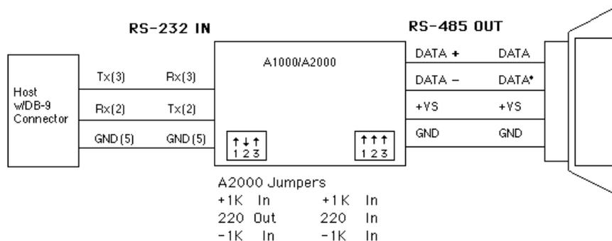
NOTE: The last module in an RS-485 string must be terminated with a 220Ω resistor between DATA and DATA\* as close to the terminals as possible.
