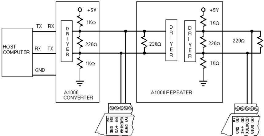
Figure 2. RS-485 biasing & termination resistors.
