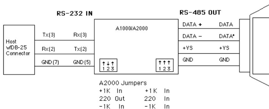
NOTE: The last module in an RS-485 string must be terminated with a 220Ω resistor between DATA and DATA\* as close to the terminals as possible.
