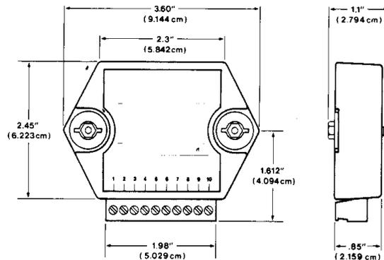
**NOTE:** Spacing for mounting screws = 2.700" (6.858 cm).
